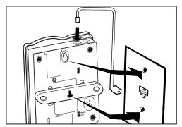
Figure 7 - Wall mounting installation
